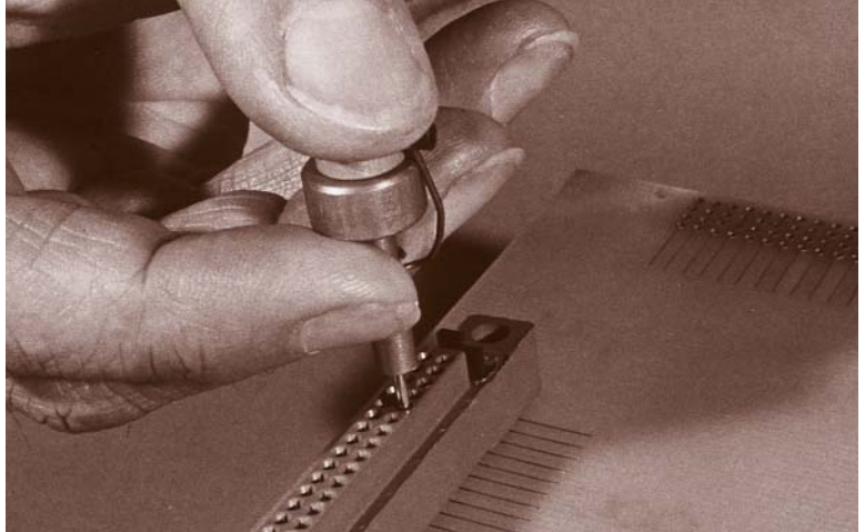
SEAT PLUNGER AND REMOVE CONTACT AND TOOL
