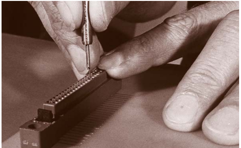
SEAT CONTACT WITH INSERTION TOOL
