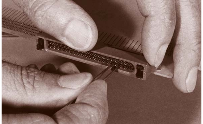
REMOVE DAMAGED CONTACT
